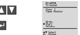
This is the default setting. Refer to chapter 7 on page 17 for other types of connection. If the DUT has been connected to the test socket. safety class recognition is performed (SC I or SC II). Otherwise, the safety class must be specified manuallv.
