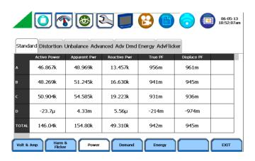
Power type parameters available in the MAVOWATT 2XX are: Watts, VA, VAR, Power Factor, Displacement Power Factor, Demand (Active, VA, VAR), Energy (WHr, VAHr, VARHr). The MAVOWATT 270 and MAVOWATT 270-400 add Forward and Reverse energy parameters.
