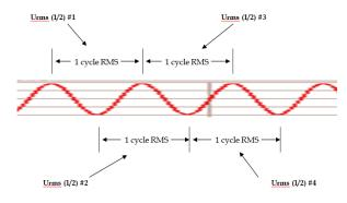
If a trigger occurs, data is stored to memory in accordance with the RMS Summary and Waveform (# of cycles recorded) settings entered during setup. Like other GOSSEN METRAWATT products, new MAVOWATT series detects and records current RMS events in the same manner as voltage. Please see the instrument user's guide for further details.
