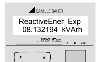
Screen 16: Reactive energy ( \int Q_{out} )
