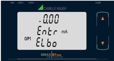
Pressing the “
