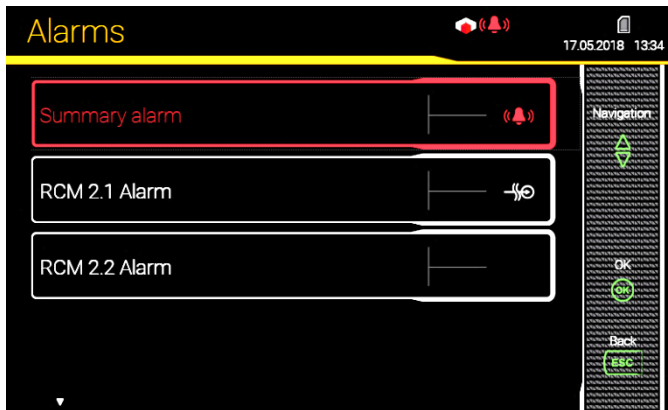
Device with RCM module: Alarm via local GUI
